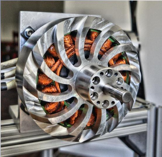
Figure 2: TFT 10 kW Halbach UHEHM1 Motor
